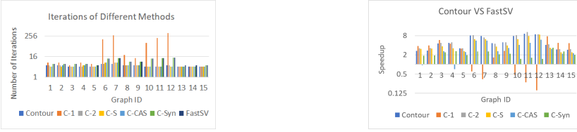
(a) Number of iterations of our different variants of Contour algorithm and FastSV algorithm for both real-world and synthetic graphs (one locale). (b) The performance of our Contour algorithm and its variants compared with the FastSV algorithm for both real-world and synthetic graphs (one locale).
